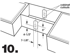
To vent through the roof with 7" round vent, mark 4-1/2" and 5" in from back wall along the centerline on underside of cabinet. Use these points as centers to draw 7-1/8" circles on underside of cabinet. Use a saber saw to cut the openings for the ventwork. Repeat for the underside of the top of the cabinet. This will create slotted openings which makes it easier to install the vent system.
